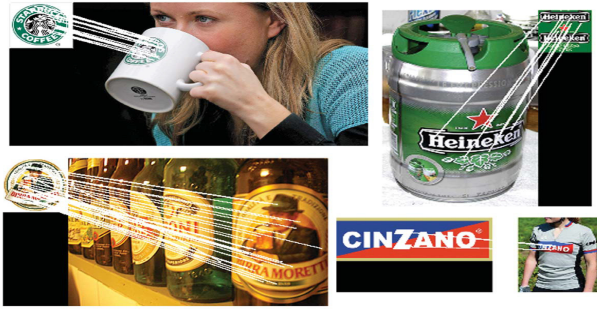
Fig.10. Some examples of logo detection results. (a) Examples of matching in case of partial appearance, perspective transformations, and low resolution. (b) Examples of matching in case of deformations. The default parameters used in these experiments correspond to \alpha = \beta = 0.1 , N_r = N_a = 8 , and \tau = 0.5 .
